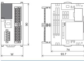
External color: Munsell 0.6B7.6/0.2 Unit: mm 35 mm width DIN rail can be installed
