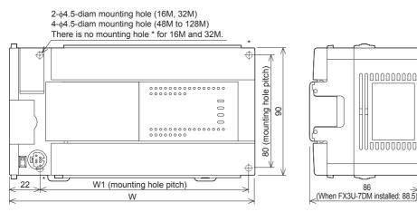
External color: Munsell 0.08GY/7.64/0.81 Top cover: Munsell N1.5 Unit: mm The terminal block uses M3 terminal screws 35 mm width DIN rail can be installed
