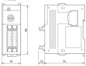
External color: Munsell 0.08GY/7.64/0.81 Unit: mm 35 mm width DIN rail can be installed
