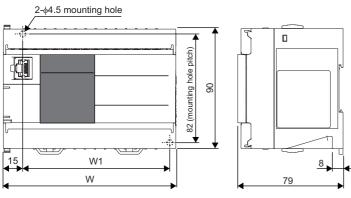
External color: Munsell 0.6B7.6/0.2 Unit: mm The terminal block uses M3 terminal screws. A 35-mm width DIN rail can be installed.
