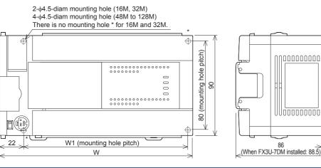
External color: Munsell 0.08GY/7.64/0.81 Top cover: Munsell N1.5 Unit: mm The terminal block uses M3 terminal screws 35 mm width DIN rail can be installed
