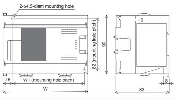
External color: Munsell 0.6B7.6/0.2 Unit: mm The terminal block uses M3 terminal screws A 35-mm width DIN rail can be installed
