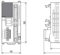
External color: Munsell 0.6B7.6/0.2 Unit: mm 35 mm width DIN rail can be installed
