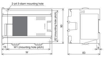
External color: Munsell 0.6B7.6/0.2 Unit: mm The terminal block uses M3 terminal screws 35 mm width DIN rail can be installed
