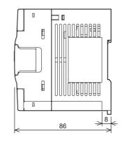
External color: Munsell 0.08GY/7.64/0.81 Top cover: Munsell N1.5 Unit: mm The terminal block uses M3 terminal screws 35 mm width DIN rail can be installed
